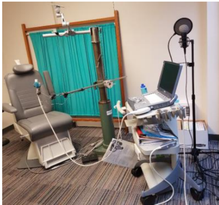
Figure 3. Ultrasound image acquisition system used in speech analysis. The system is also configured with a microphone and head-transducer stability system. The copyright for the ultrasound and head-transducer support system picture belongs to the author of this article, Khalid Al-hammuri [5].
